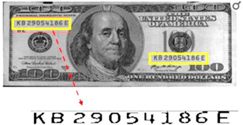
Most conventional sensors for banknote recognition are visible-light line sensors, such as contact image sensors (CIS). Such sensors mostly obtain color or black-and-white images and are used for the typical process flow of preprocessing, feature extraction, classification, and verification.
